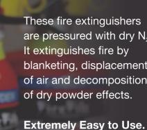
These fire extinguishers are pressured with dry N<sub>2</sub>. It extinguishes fire by blanketing, displacement of air and decomposition of dry powder effects.
